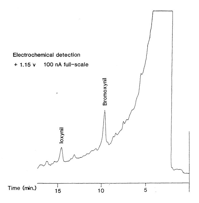
HPLC separation of a spiked river water (0.1  $\mu g \Gamma^{1}$ ) extract
