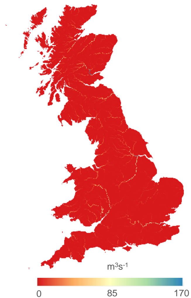
Figure 6.2 Mean flow for Great Britain in a 1 km grid estimated by the G2G model using gridded rainfall data and MORECS evapotranspiration estimates (Bell et al., 2018).
